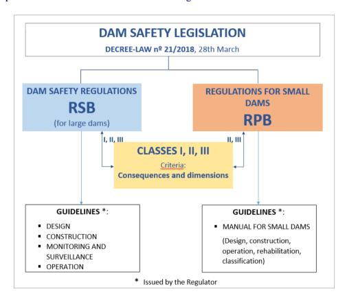
RSB applies to "large dams" dams, defined on the basis of a dimensional criteria of dam height greater than 15m, and additionally of reservoir capacity greater than 1.000.000 m3 (1 hm3) with height greater than 10m. This RSB definition of "large dam" is broadly based on the ICOLD definition.
